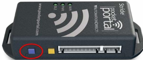
The BLE (Bluetooth Low Energy) LED on the Pocket Portal will blink to indicate that the device is in advertising mode and ready to accept connections.
