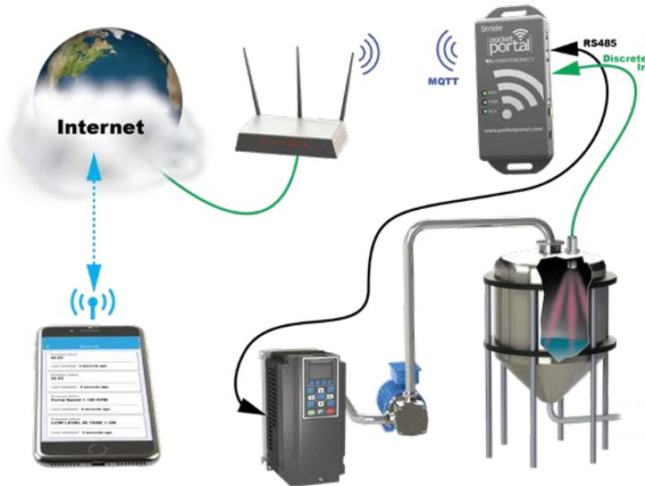
As shown in the example above the *STRIDE* Pocket Portal will connect a Modbus RTU slave device, digital I/O or analog inputs to the cloud-based Pocket Portal platform to allow remote data monitoring and data logging. The Pocket Portal connects to its cloud platform via the Internet using a locally-provided Wi-Fi access point, so no network wiring to the machine is necessary.
