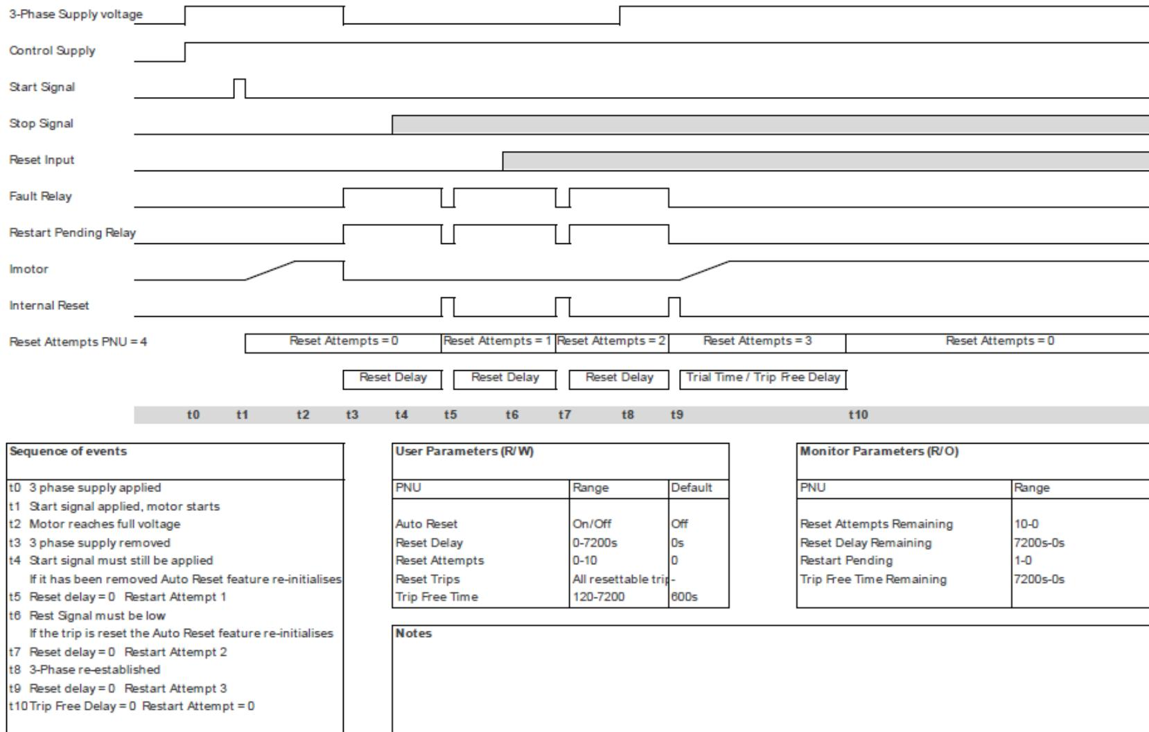
Fig 4 : Auto Reset - Three Wire - Control Supply Loss
