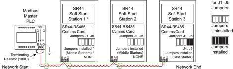
\* The 'Network Start' terminating resistor is installed at the PLC, and Station 1 is jumpered as a 'Middle Starter'.
