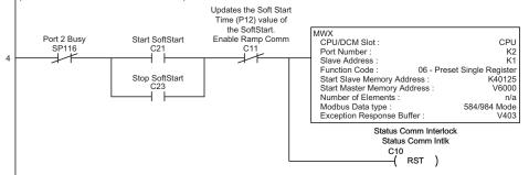
This rung will reset the Status Comm Interlock if no attempt is made to write to the soft starter. This will allow rung 3 to read the status again. Status will be read continuously from the starter, and writes will be done by excepton, that is, when the user causes it.
