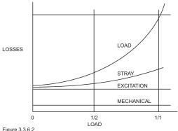
Motor Efficiency/Loss Characteristic
