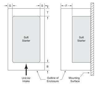
Minimum Clearance for Heat Dissipation
