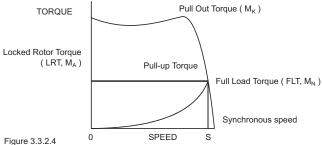
Torque/Speed Curve – High Starting Torque
