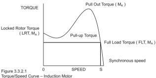
Figure 3.3.2.1: Torque/Speed Curve - Induction Motor
