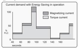
The calculations to cover all the likely or possible conditions would be laborious. An empirical method for arriving at a usefully realistic estimate has been devised. Used with a proper sense of engineering circumspection, the tables in Section 3.4.6 allow a user to gain a reasonably close estimate of the savings to be achieved within the motor by using the SR44 optimizing Soft Starter. The method does not include any additional savings and benefits conferred by other sources, such as:
