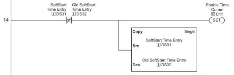
This rung will be activated, until DS31 is equal to DS41, which is the Received value from the unit. When equal, the sequence is reset.
