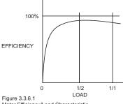
Motor Efficiency/Load Characteristic
