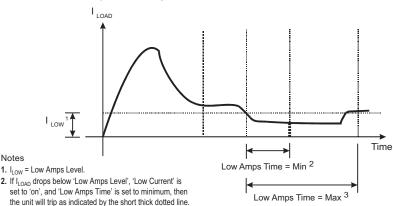
3. If 'Low Amps Time' is set to maximum and  $\rm I_{\rm LOAD}$  rises above 'Low Amps Level' before 'Low Amps Time' has elapsed, then the unit will not trip.
