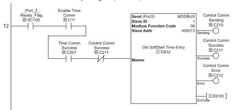
When both comm instructions have successfully operated, this rung will reset the communication bits and allow the comms to restart.
