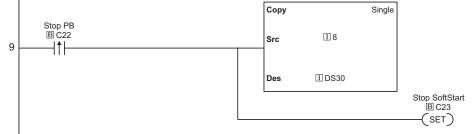
When the "Stopping" or "Stopped" bits (read from the unit) turn on, the "Stop" sequence is reset.
