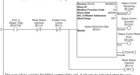
This rung will be used for Start/Stop control of the unit. It will only be activated when the user activates the Start and Stop inputs, which will send a value of "7" (Start) or "8" (Stop), contained in DS30, to the "Command Register" (P124) of the unit.
