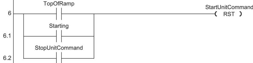
*This rung, controlled by “StopUnit” input (usually a pushbutton input to the P3) activates the “Stop Unit” sequence by setting the Bool tag “StopUnitCommand”. Then a value of 8 (“Bus Stop”) is written to tag “P124 Starter Control”. Again, writing will begin until status bits reflect the desired response. Then the sequence resets.*
