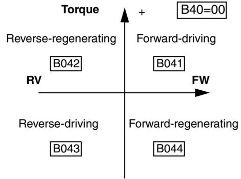
The terminal selection mode (B040=01) uses two intelligent inputs [TRQ1] and [TRQ2] for the binary-encoded selection of one of the four torque limit parameters B041, B042, B043 and B044.
