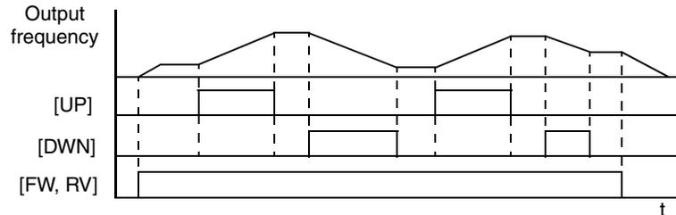
It is possible for the inverter to retain the frequency set from the [UP] and [DWN] terminals through a power loss. Parameter C101 enables/disables the memory. If disabled, the inverter retains the last frequency before an UP/DWN adjustment. Use the [UDC] terminal to clear the memory and return to the original set output frequency.
