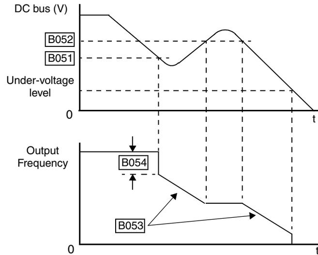
**NOTE:** (1) Be sure to set the *over-voltage threshold* greater than the *DC bus voltage trigger level* ( $B052 > B051$ ) for proper operation.
