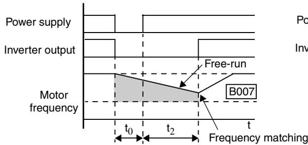
Motor frequency > B007 value at t<sub>2</sub>
