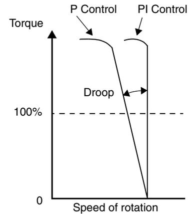
The proportional gain  $K_{pp}$  value determines the droop. Set the desired value using parameter H052. The relationship between the  $K_{pp}$  value and the droop is shown below:
