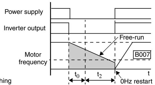
Motor frequency < B007 value at t<sub>2</sub>
