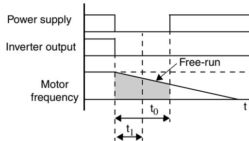
Inverter trips when  $t_0 > t_1$
