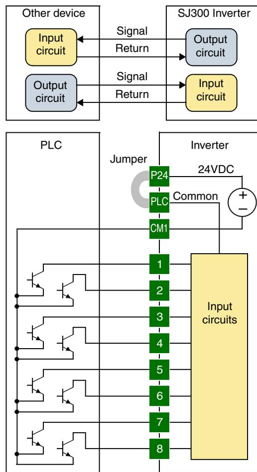
**Example Wiring Diagram**
