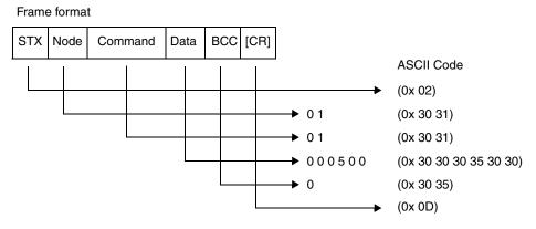
The block check code is computed by using the ASCII codes (shown above) and applying eXclusive OR (XOR) operations. Beginning with the first pair of bytes, the result of their XOR result is then used in an XOR operation with the third byte, and so on. For this example, the BCC calculation is shown below.
