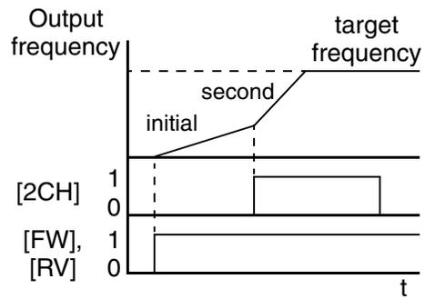
In the graph shown above, the [2CH] becomes active during the initial acceleration. This causes the inverter to switch from using acceleration 1 (F\_02) to acceleration 2 (A\_92).
