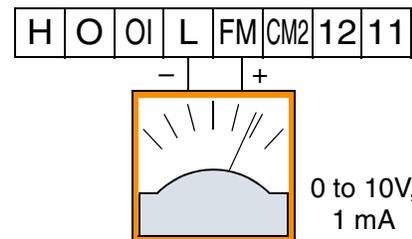
The signal characteristics of terminal [FM] in PWM configuration is shown below:
