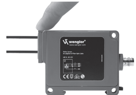
Fig. 8: Connecting the plastic fibre-optic cable
