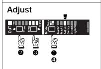
The detection zone can be set manually, or when set by the teach function, can be manually fine adjusted. All activated functions (except delay and stretch) are in operation, and the output switched.
