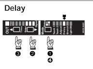
Switching of the output is delayed by the set time. In this way, short-term disturbances can be suppressed. All activated functions (except delay and stretch) are in operation, and the output switches.
