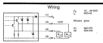
pin assignment (view onto device)
