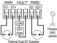
\*Fault Contact opens when in a faulted state
