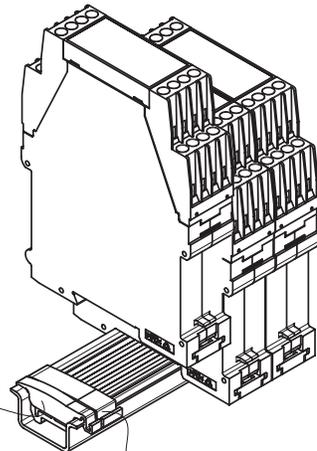
Safety cap on both sides tight to the carrier profile
