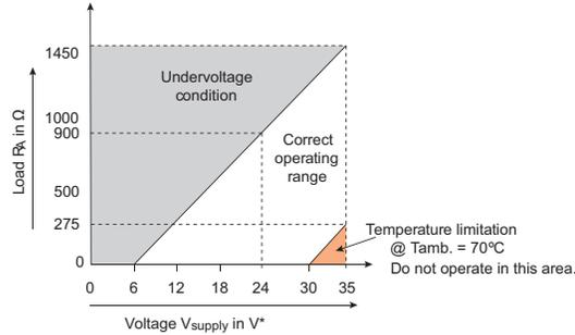
SC6-4102, -4112 Output Load Derating @ Tamb. = 60°C . . . No limiting issues within operating range
