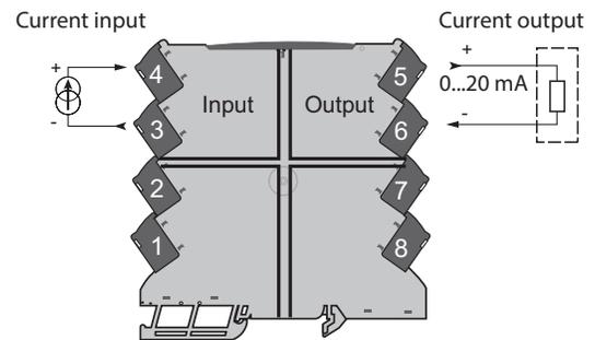
**Bipolar Input to bipolar output wiring set-up:**
