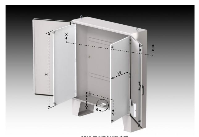
DEAD FRONT PANEL SIZE: H = DOOR OPENING HEIGHT - 1.50" W = (DOOR OPENING WIDTH / 2) + 0.13"
