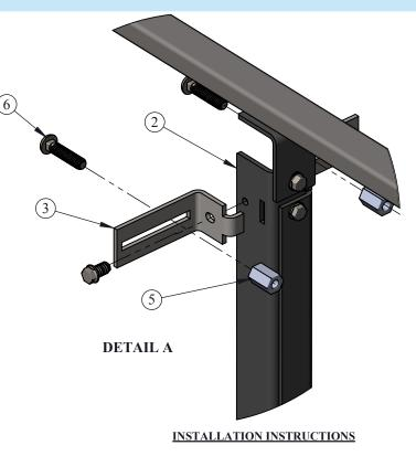
**STEP 1**: FIRST INSTALL CENTER PANNEL SUPPORT (ITEM 2) IN THE ENCLSOURE USING HARDWARE INCLUDED IN BOLT PACK **102027** (SEE **CENTER PANEL SUPPORT INSTALL MANUAL** IF NEEDED).
