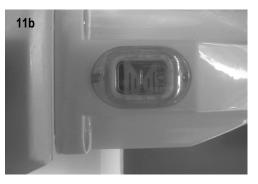
11c. For long rope spans >50m. it advised to balance the system by making turns to the Left and Right Tensioner/Grippers in turn whilst checking the rope tension setting in each switch viewing window.
