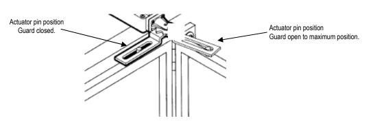
Check closed and open positions before permanently fixing the pin.
