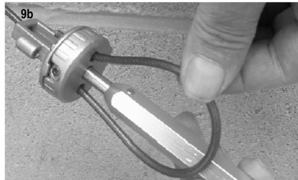
10a. The rope is then pulled by hand through the Tensioner / Gripper to take up any slack rope before final locking.
