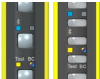
FIG. 8A: LED INDICATORS ON SENDER UNIT (30 MM AND 14 MM RESOLUTION)
