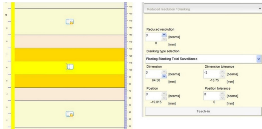
Figure 60 - Floating Blanking with total surveillance
