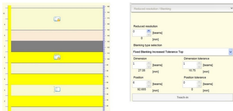
Figure 59 - Fixed Blanking with increase tolerance
