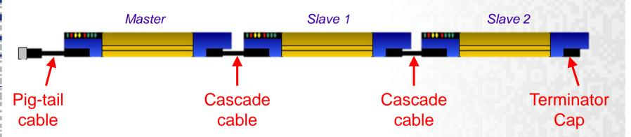
The Cascade connection can be made using 2 or 3 Light Curtain (standard model), also with different length and different resolution (please refer to the User Manual).
