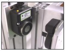
MGL shown in CLOSED position, lock energised. Steady Green LED indication.
