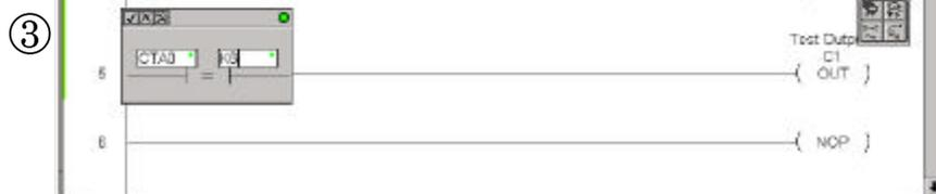
Next, move the cursor to the end of the pasted rung. With the cursor over the **C1** output element, double click with your mouse. This opens the window for editing the output coil. Change it to **C2**.
