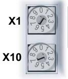
Modbus Station Rotary Switch
