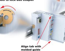
Where applicable, rotate Locking Wheel to unlock Bus Coupler
