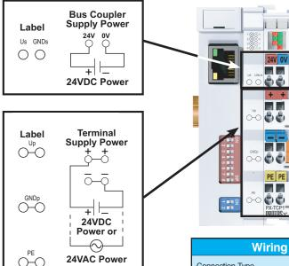
Wire connections are made through spring clamp style terminals. The terminals are designed for a singleconductor solid or stranded wire. Wire connection is made by firmly pushing the screwdriver into the screwdriver slot, inserting the wire into the wire slot and removing the screwdriver, locking the wire into position.
