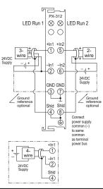
Two-channel, -10 to +10 VDC Analog Input Terminal
