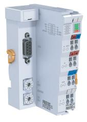
The PX-MOD Modbus RTU/ASCII Slave Bus Coupler allows connection of up to 64 terminals per assembly, 255 terminals total, in a Modbus RTU/ASCII serial network. The PX-MOD communicates using high-level Modbus commands and automatically assigns Modbus addresses for inputs and outputs. The maximum amount of data is 512 bytes of input data and 512 bytes of output data, with up to 1020 inputs, 1020 outputs, 256 analog inputs and 256 analog outputs, when using bus expansion.
