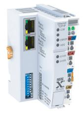
The PX-TCP2 Modbus TCP Server Bus Coupler allows connection of up to 64 terminals in a Modbus TCP network. The PX-TCP2 communicates using high-level Modbus commands and automatically assigns Modbus addresses for inputs and outputs. The maximum amount of data is 512 bytes of input data and 512 bytes of output data, with up to 512 inputs, 512 outputs, and 128 analog inputs or outputs.
