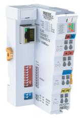
The PX-TCP1 Modbus TCP Server Bus Coupler allows connection of up to 64 terminals per assembly, 255 terminals total, in a Modbus TCP network. The PX-TCP1 communicates using high-level Modbus commands and automatically assigns Modbus addresses for inputs and outputs. The maximum amount of data is 512 bytes of input data and 512 bytes of output data, with up to 1020 inputs, 1020 outputs, and 128 analog inputs or outputs, when using bus expansion.
