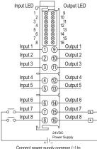
Connect power supply common (–) to same common as terminal power bus
