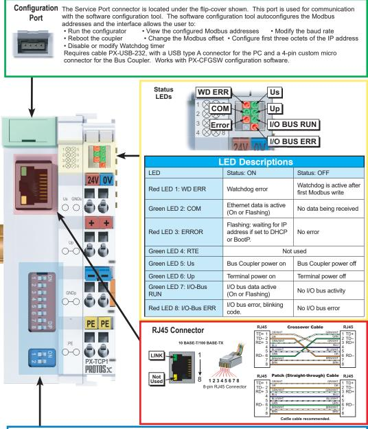
Address Selection DIP Switches DIP Switches
