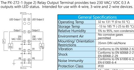
Note: Terminal PX-908 is recommended to isolate terminal power or use PX-970 to supply and isolate power.
