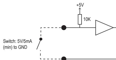
Figure 3 – Simplified Battery Remote On/Off Circuitry
