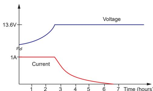
Figure 4 – Battery Charge Characteristics
