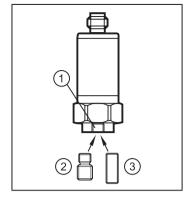
▶ Tighten the sensor with a tightening torque of 8 Nm.
