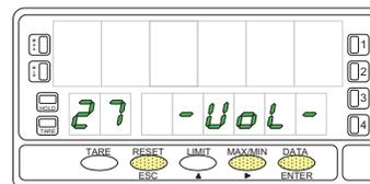
**Selection of the tank's shape.** There are 5 options: **-no-** to disable this facility, **-tYP 1-** for spherical shape, **-tYP 2-** for horizontal cylinder, **-tYP 3-** for horizontal cylinder with end caps and **-tYP 4-** for conical bottom vertical cylinder.
