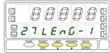
**SILO:** The silo shape (tYP 4) is a combination of three parts and requires **three diameters and three lengths** to be programmed. You may have a tank that is composed of only one or two of the parts in which this shape is divided, to overcome this situation, the length of the missing parts should be programmed to zero. The last phase of this routine is to set the decimal point of the display.
