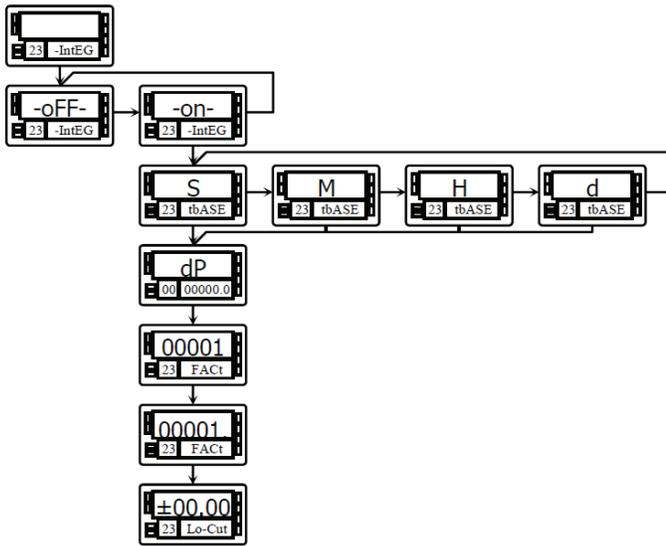
The instrument provides an 8 digit counter (or 7 digits with negative sign) that can be used to accumulate readings in totalizing+batch applications (logic function nº 30 at the rear connector) or to integrate the instantaneous reading using a time-base.
