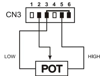
Note: A jumper wire from pin 6 to pin 3 needs to be installed when wiring a potentiometer. The low potentiometer wire and jumper wire will both terminate in pin 3 of CN3.
