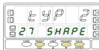
After selecting the tank's shape, it is necessary to enter the **dimensions of the tank**. The figure shows the phase corresponding to the programming of the diameter D1.
