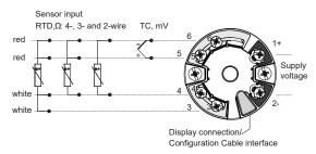
Note: In the event of a thermocouple (TC) measurement, a 2-wire Pt100 RTD can be connected to measure the reference junction temperature. This is connected to terminals 4 and 6.
