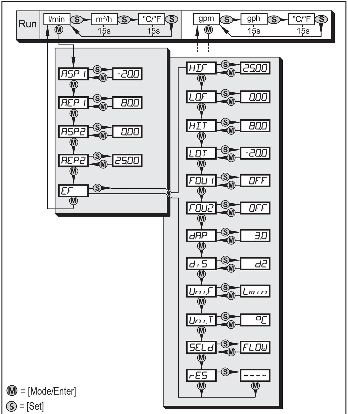
In the Run mode, different display units are accessible (depending on the setting of the parameters [SELd], [Uni.F] and [Uni.T], → 10.4).
