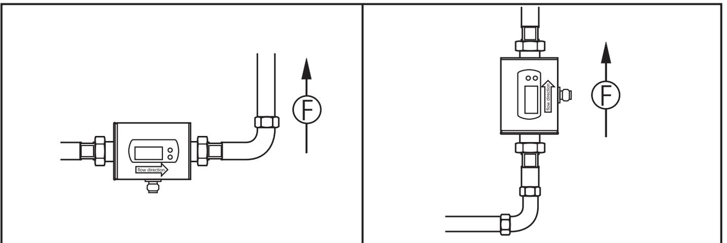
S = disturbance; D = pipe diameter; F = flow direction
