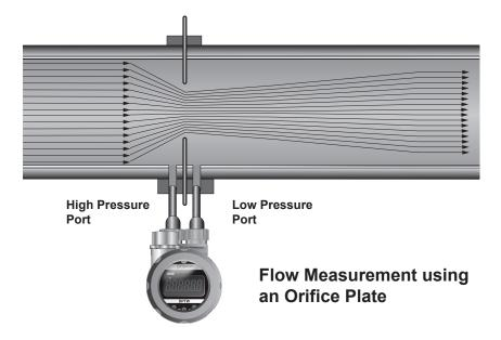
Flow rate is calculated by measuring the differential pressure across an orifice plate. The DPTW will be using the orifice plate manufacturer's data of maximum flow rate with corresponding differential pressure drop.
