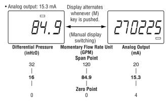
The momentary flow rate Dx at the measured differential pressure of 16 inH2O (40% F.S.) is calculated by the following formula:
