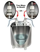
Suggested assembly. 8mm diameter GWR-P240 through GWR-P1600 probes can be used with BSPBX-12-W cable gland and CLC-ACC1 wiring kit. Can be mounted through tank hole with included nut or without the included nut when installed in a 1/2" NPT tank flange.
