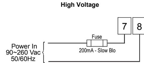
Note: The installation of fuse is optional, depending on level of protection required.
