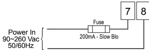
Note: The installation of fuse is optional, depending on level of protection required.
