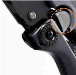
Ratchet (with emergency release) to ensure completed crimps
