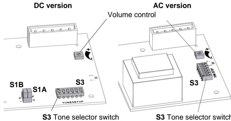
**S1B:** Selection of control voltage polarity for C1 and C2 (external control)
