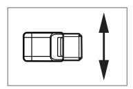
The objects to be detected are to move transversally to the lens of the sensor. In case of other directions of movement it should be tested for operation of the switching function.
