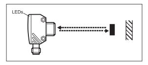
Align the diffuse reflection sensor to the object to be detected and secure it to a bracket.
