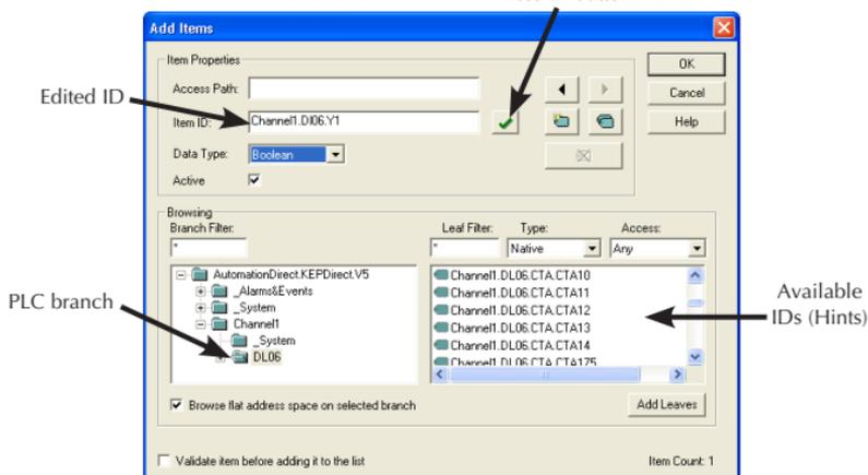
Item ID window. Edit the ID by removing "Hints" and by typing the correct address. In this case, we are using the address Y1. Clicking on the ✓ button will test the ID. If the ID is not correct, an error message window will pop-up. If the ID is correct, the **Data Type** will be automatically chosen.
