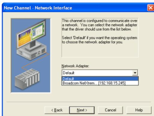
Click on the down arrow to open the drop down list. Select the Ethernet **Network Adapter** that you would like to use to connect to the ECOM module. This list displays any detected network cards from your computer. Either select the adapter you wish to use or select **Default** and allow the operating system to select the adapter.
