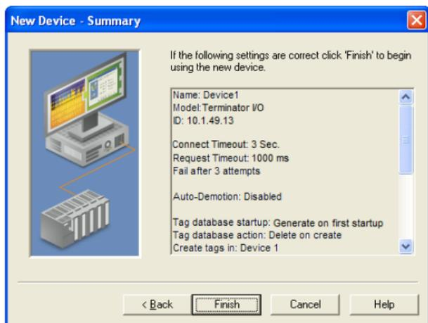
Review the summary and click on **Finish** to complete the device setup. If server's tag database was set to automatically generate, then the server will attempt to connect to the device and create a tag database using the device's configuration. If the database creation was set to manual, refer to the "Creating Tags" section for information on adding tags to the project.
