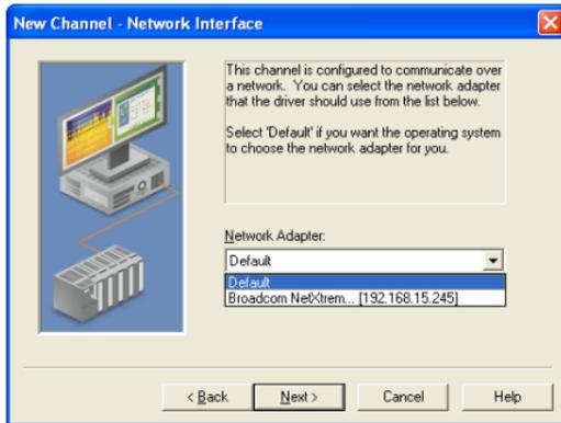
Click on the down arrow to open the drop down list. Select the Ethernet **Network Adapter** that you would like to use to connect to the EBC module. This list displays any detected network cards from your computer. Either select the adapter you wish to use or select **Default** and allow the operating system to select the adapter.
