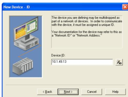
Enter the IP address of the ECOM module you wish to monitor. It is important that the IP address is typed correctly and that it corresponds to the device being installed. Click on the **Next** button to continue with the device installation.
