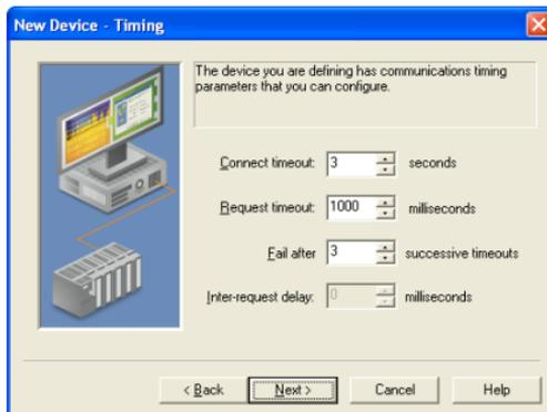
This screen provides three different communication settings for the device being installed. The following list explains the purpose of each available setting.
