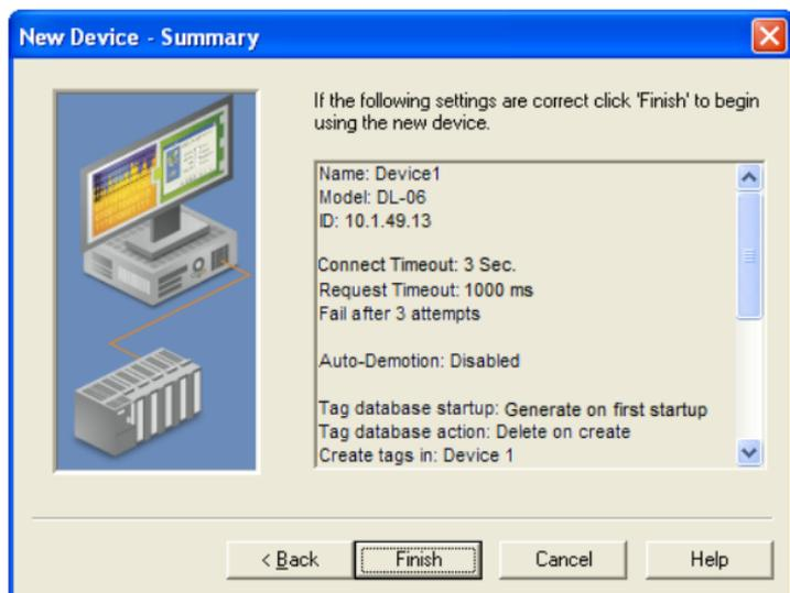
Review the summary and click on **Finish** to complete the device setup. If server's tag database was set to automatically generate, then the CSV file selected in the previous step will be used to create the database as soon as the device setup is completed. If the database creation was set to manual, refer to the "Creating Tags" section for information on adding tags to the project.
