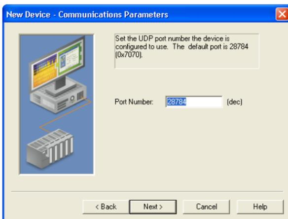
This parameter is used to select the port number to be used by the driver for communicating with the remote device. The default value is 28784 (0x7070). Legal port number values are between 0-65535.
