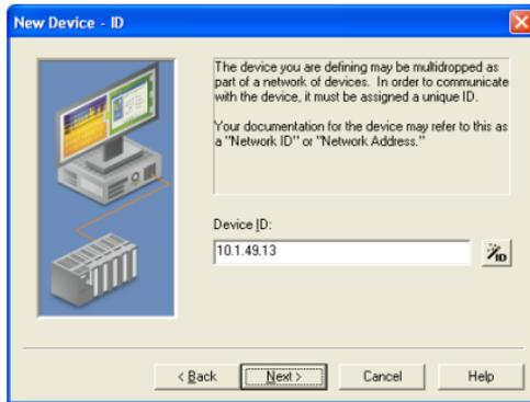
Enter the IP address of the EBC module you wish to monitor. It is important that the IP address is typed correctly and that it corresponds to the device being installed. Click on the **Next** button to continue with the device installation.
