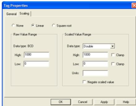
Selecting either **Linear** or **Square Root** will enable the scaling parameters. The **Raw Value Range** allows you to specify the range of raw data from the device. The valid range is dependent upon the data type of the raw tag value. If, for example, the data type is set to Short, the valid range of the raw value would be -32768 to 32767. The raw high range must be greater than the raw low range.
