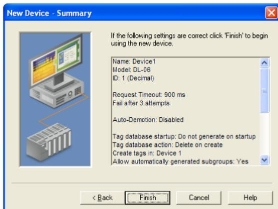
Review the summary and click on **Finish** to complete the device setup. If server tag database was set to automatically generate, then the CSV file selected in the previous step will be used to create the database as soon as the device setup is completed. If the database creation was set to manual, refer to the "Creating Tags" section for information on adding tags to the project.
