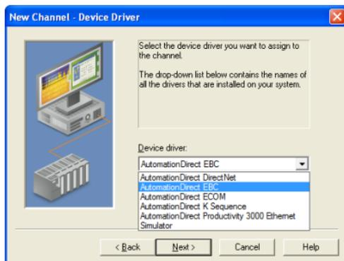
The **Device Driver** window will open. The arrow to the right side of the name provides a drop down list of device drivers that are available on your system. From this list, select **AUTOMATIONDIRECT EBC**. After selecting the device driver, click on the **Next** button to go to the next step.
