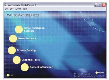
The AutomationDirect installation window will display all software options available on this CD. To install DataWorx WinPLC select the INSTALL PURCHASED SOFTWARE option. This selection opens the Product Key window shown below.
