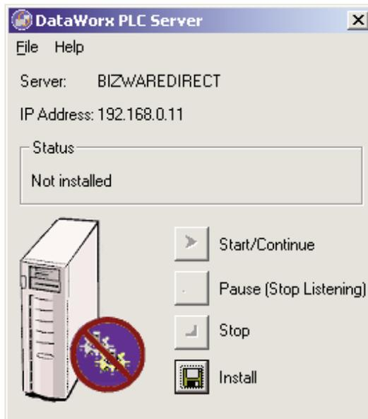
Click **INSTALL**. The DataWorx PLC Server window will update and display the Server Status as “Installed, Stopped.”
