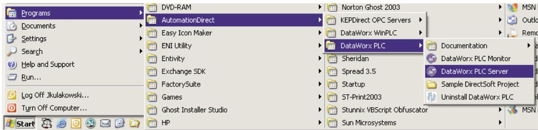
The DataWorx PLC Server window will open. If the Server has already been installed, the Server Status will display as “Installed; Stopped.”
