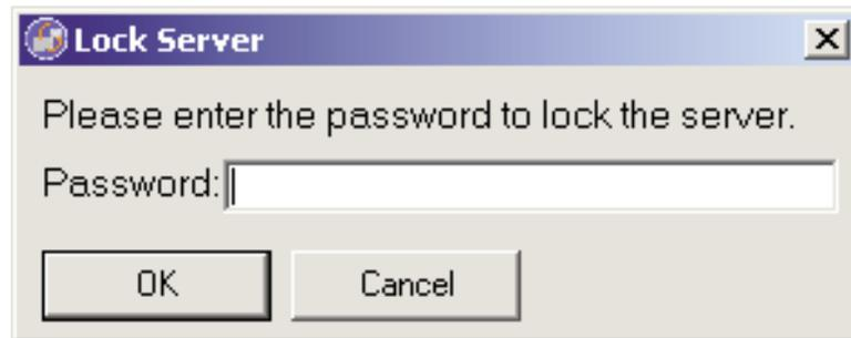
Enter a lock Password, and click **OK**. If successful, the Status section will display a Locked status:
