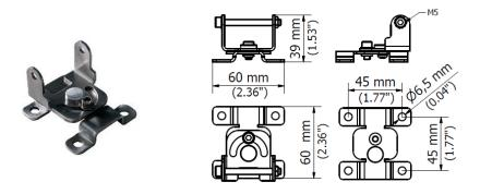
cod. **SRQFX01** Bracket-set in stainless steel Adjustment left and right rotation  $A = +90^{\circ} /- 90^{\circ}$  Adjustment front and back inclination (B) =  $+90^{\circ} /- 90^{\circ}$
