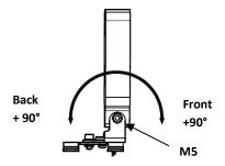
**B.** For side left adjustment: untighten the M5 bolt on the rear head, choose the position, and tighten again.
