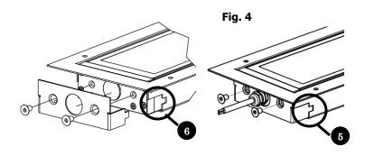
**Fig.4** Mount the Two closing part making sure that side pins 6 and 6 have properly inserted into frame slots. Screw M6x10 screws to tighten closing parts to the fixture.
