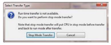
Stop Mode transfers allows the user to transfer any and all ladder, Tag database and configuration changes to the CPU.
