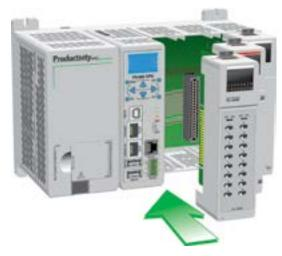
4. Connect appropriate wiring to power supply and I/O, a P3-01AC and P3-08TAS in this example.
