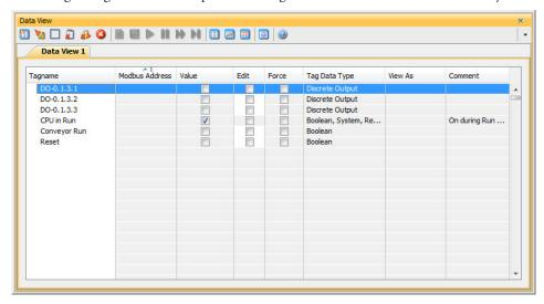
program interface while in "Monitor" mode, as long as the "Forceable" box has been checked in Tag Database. I/O may also be directly forced in I/O View by clicking on individual I/O points.
