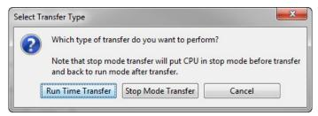
The above dialog is accessed two ways: (only when CPU is online AND in run mode) Perform either of the following to transfer project to the CPU:
