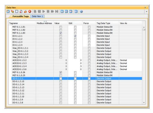
From either of these windows you have the option to select the check box in the Force column. When this box is checked and the row is selected (selected rows show high-lighted blue) and you select the Send Edit(s) button, the current row(s) will be forced.
