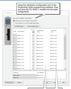
The "Under Range Error" bit for each channel activates for a signal around 0mA ± offset error.
