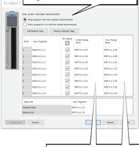
The "Under Range Error" bit for each channel activates for a signal around 0V ± offset error.
