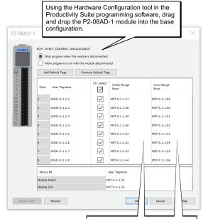
The "Under Range Error" bit for each channel activates for a signal around 0mA ± offset error.
