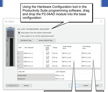
The "Under Range Error" bit for each channel activates for a signal aat range minimum ± offset error (-9.999 V, -4.999 V, 0V amd 0mA).
