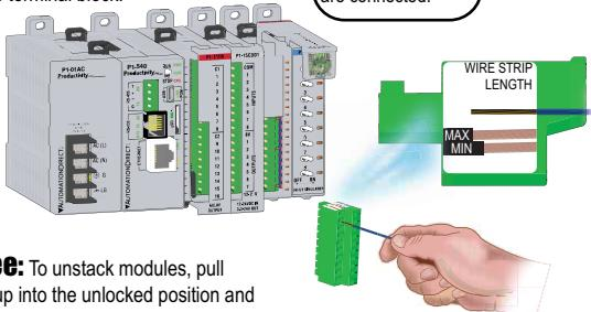
**Step Three:** To unstack modules, pull locking latch up into the unlocked position and then pull modules apart.
